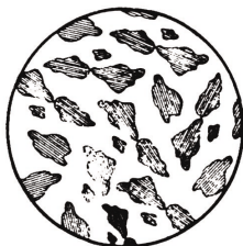
Microphotograph of fused flux shows uniformity of particles.
