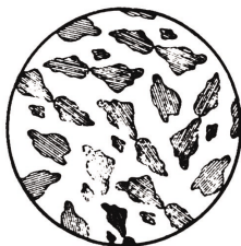
Microphotograph of flux shows mesh size uniformity of bonded, large particles.
