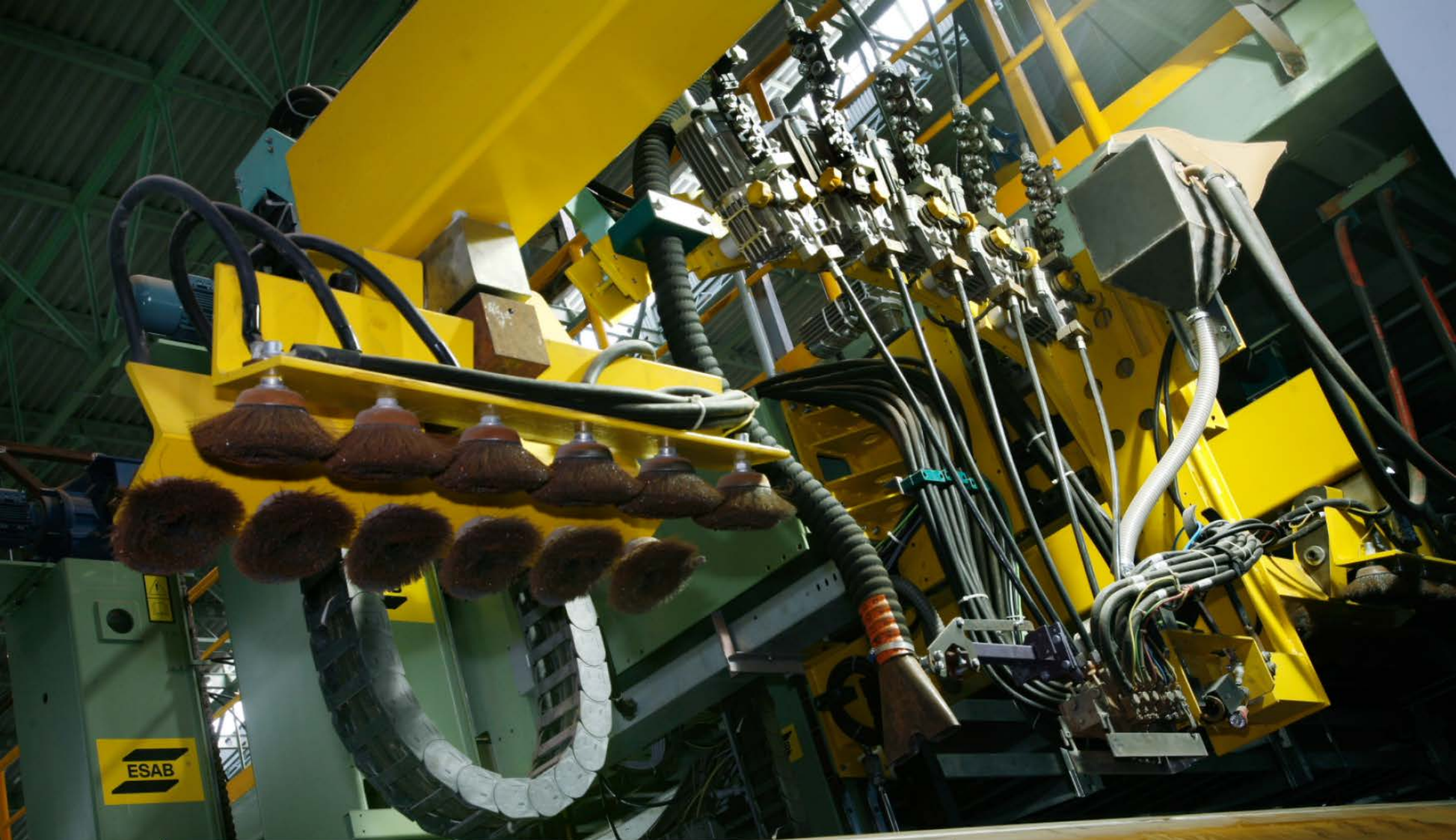
External head and grounding system
