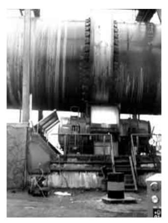
The ESAB OK 92.26 stick electrode is nickel based and is suitable for steels with limited weldability. Tyre bands and support rollers are always in need of maintenance due to spalling and cracking. The electrode is also suitable for Inconel 600, similar Inconel alloys and cryogenic steels. It's heat resistant and appropriate for welding martensitic steels to austenetic steels.
