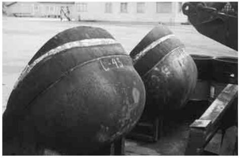
Dredger bucket. Joining new bucket lips using OK 68.82.
