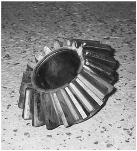
Gear drive. Rebuilding using OK 68.82.
