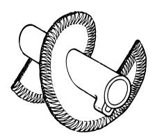
Before welding, remove defective material by gouging with OK 21.03 or by grinding. Working edges are hardfaced with wear-resistant electrodes OK 83.65 or OK 84.78, or flux-cored wires OK Tubrodur 14.70 or OK Tubrodur 15.52.
